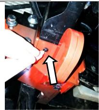
13. Using a white paint marker, mark point onto mount assembly using mounting hole in recovery point as a guide (shown).
