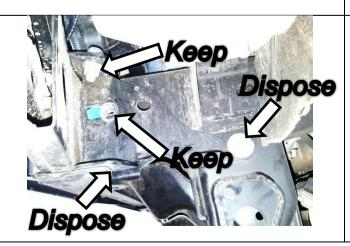
4. Remove 4x fasteners which retain outer chassis rail bracket and remove bracket.
