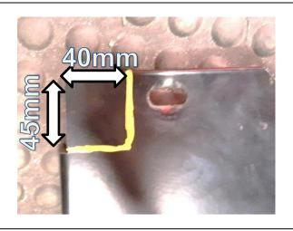
24. Mark section outlined onto flange of wing under panel as shown.
