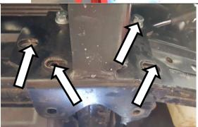
3. Remove and dispose of 4x fasteners located at front of mount assembly.
