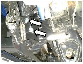
7. Position modified chassis rail bracket back onto vehicle and loosely fasten using fasteners retained from Step 4.
