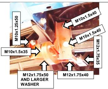
12. Position recovery point onto vehicle as shown and loosely fasten to mount assembly and chassis using 1x M10x1.5x35 bolt, 2x M10x1.5x40 bolt, 1x M10x1.25x50 bolt, 1x M12x1.75x50 bolt,
