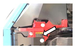
35. Position secondary load rating label on recovery point as shown.
