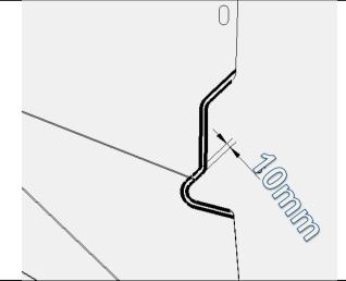
23. Using white paint marker, mark section shown onto wing under panel 10 mm offset from profile edge.
