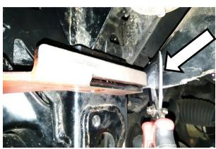
21. Trim small section of wheel arch guard using recovery point as guide as shown.
