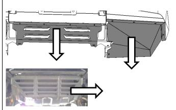
1. Remove stone guard, wing under-panel, OEM sump guard and associated fasteners and set aside for later re-use.
