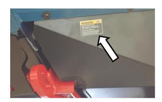
34. Position load rating label on wing under panel as shown.
