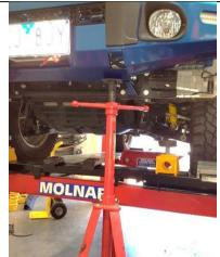
2. Position support stand as shown to support the bull bar when removing bolts from the mount assembly in the following steps.
